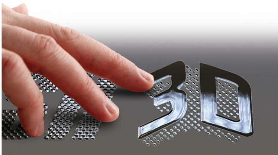
Figure 6: Dimensional UV Inkjet Special Effect
