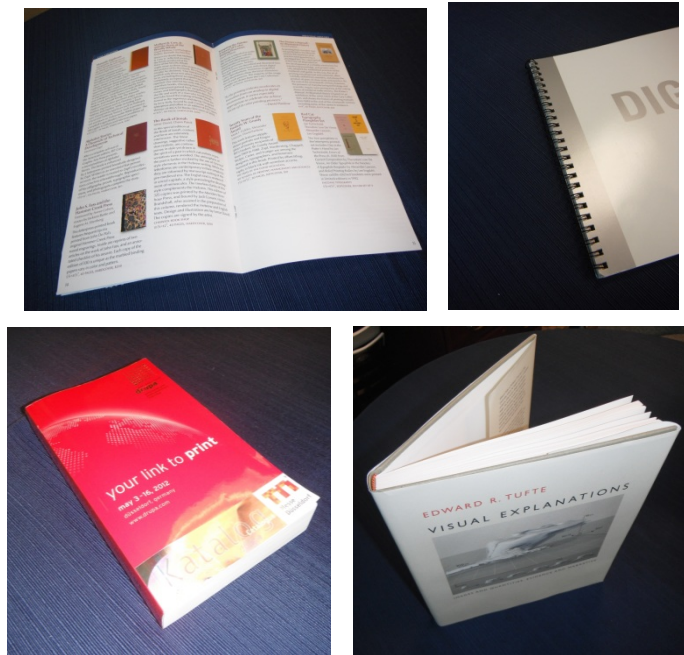
Figure 3: Binding methods of Stitching (upper left), Mechanical (upper right), Soft Cover (lower left), and Hardcover (lower right)
