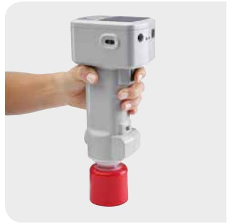
Color measurement of plastic article with spectrophotometer CM-700d (Photo: Konica Minolta)
